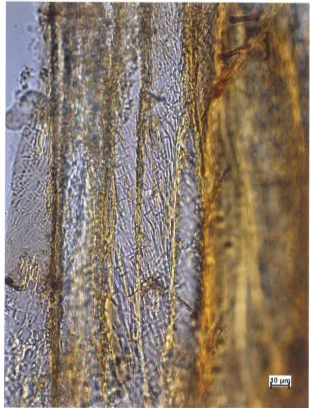
Figure 2: specimen 1; TMT Yellow Poplar, caverns of soft rot fungi, M 600:1
