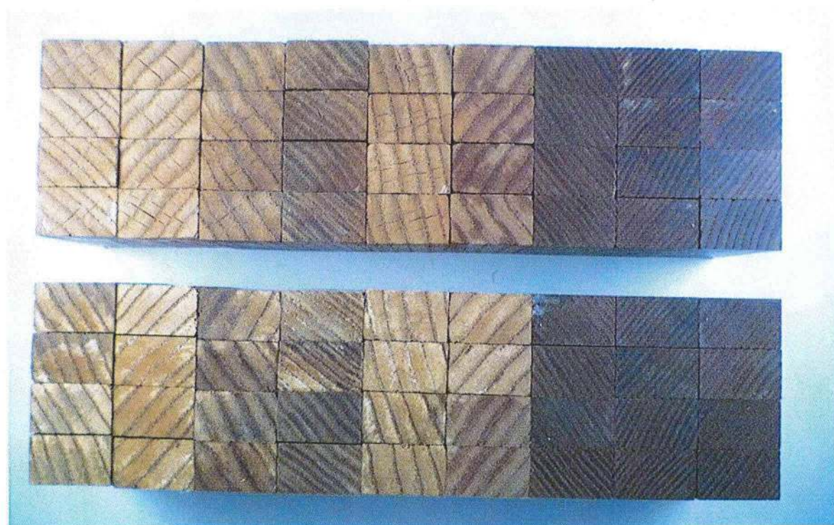
Fig. A2: specimens after the fungus test (top: Coniophora puteana , bottom: Coriolus versicolor )
